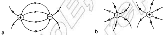
Figure 2.23 Electric fields around a pair of opposite charges, and a pair of charges with the same sign.
